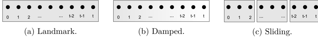
Figure 4.3: Window models visualization. The intensity of the background color represents an object’s weight.
