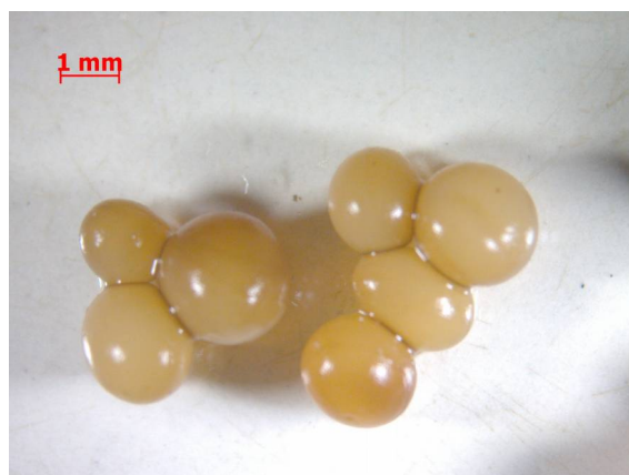
Obr. 22 Mikroperly 2% CH+5% TPP+1% HK
