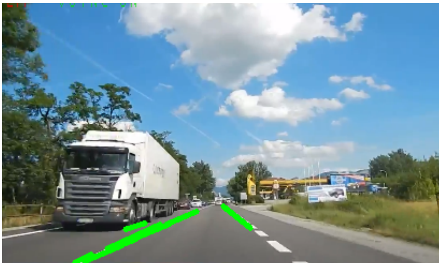
Fig. 44: Straight lanes found by the HoughLinesP algorithm
