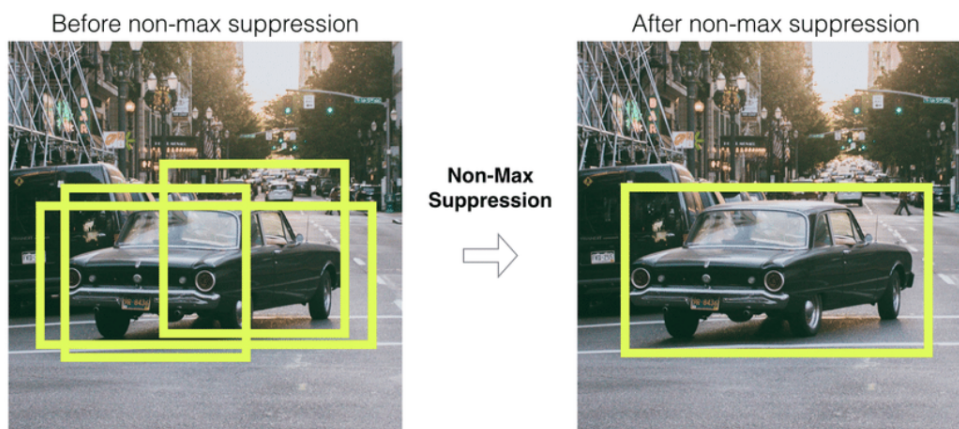
Fig. 32: Non Maximal Suppression NMS [17]
