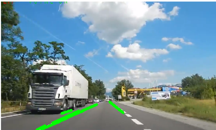
Fig. 44: Straight lanes found by the HoughLinesP algorithm
