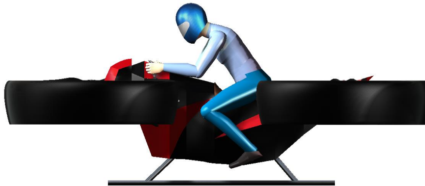
Figure 8.2 Ergonomics of the multicopter with the pilot 185 cm tall
