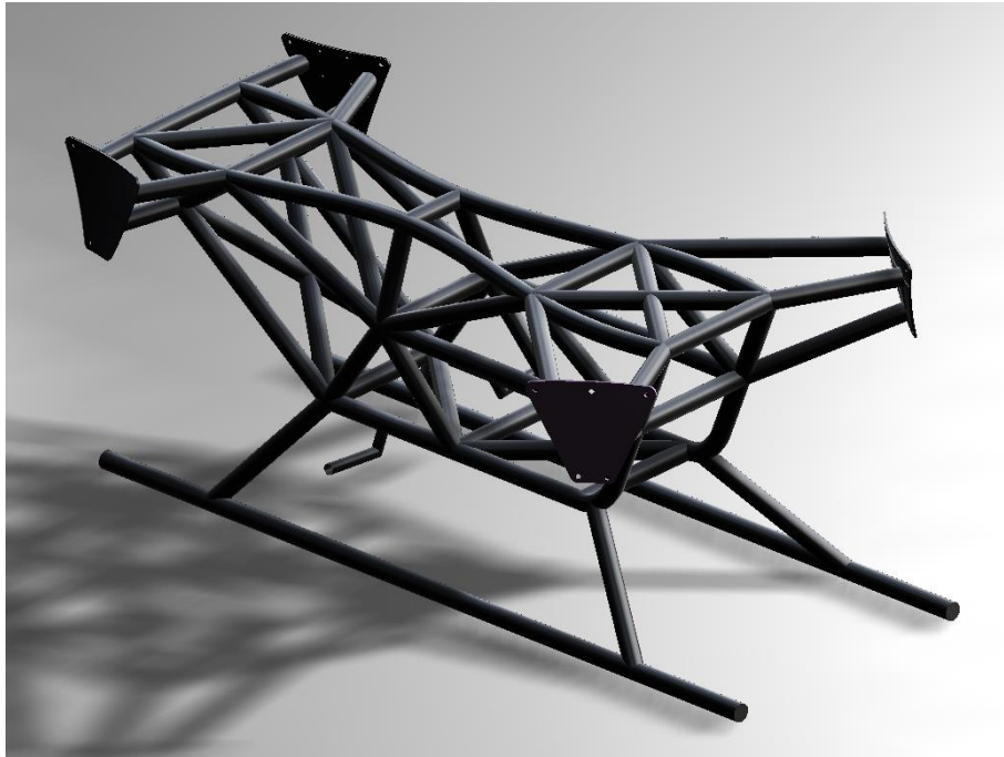
Figure 8.6 Multicopter space frame with duct connecting plates
