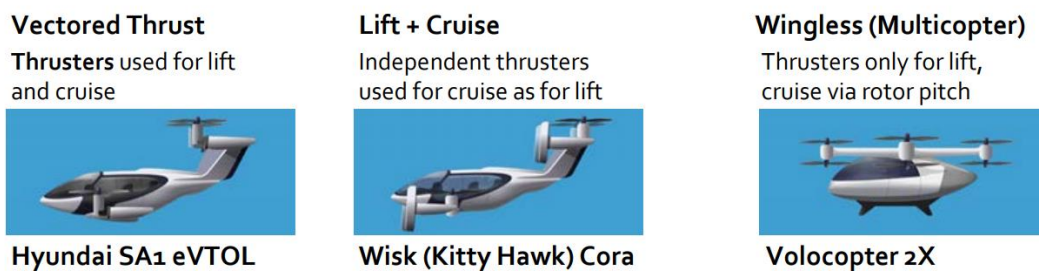
Figure 2.1 UAM types from the propulsion system perspective [3]
