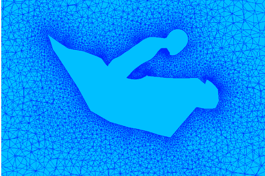
Figure 11.21 Mesh refinement around model body
