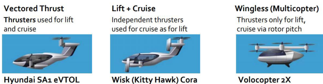
Figure 2.1 UAM types from the propulsion system perspective [3]
