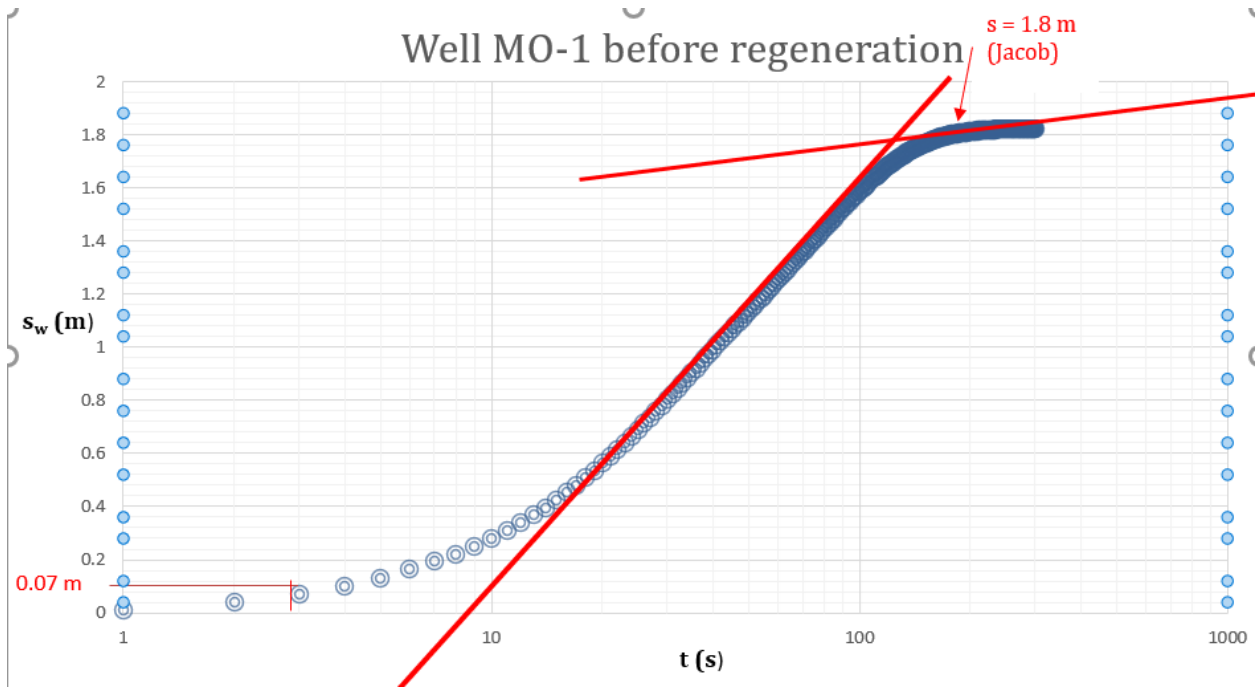
Figure 23. Representation of time vs drawdown plot of the MO-1 pumping well before regeneration.
