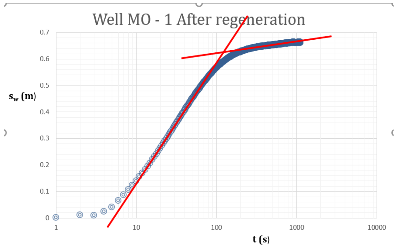
Figure 24. Representation of time vs drawdown plot of the MO-1 pumping well after regeneration.
