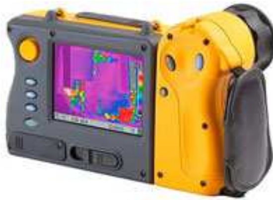
Obr. 36 Termokamera Fluke TI-55FT [24]
