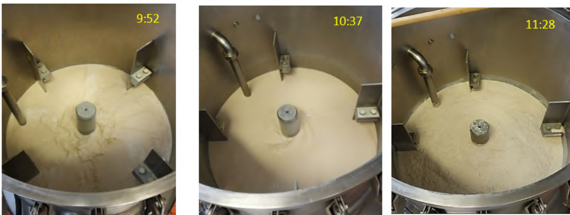
Fig. 4.12: Consistency of biomass during experiment. 9:52 – raw biomass, 10:37 – alkaline gel, 11:28 – floculated
