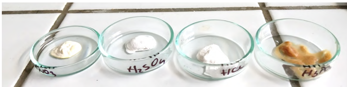
Fig. 4.17: Acid digestion with different acids. Preparation followed general procedure 3.3.2.1, biomass concentration was 38 % CDW, concentration of acid in reaction mixture was 0.4 mol/l and the mixture reacted 3 h/95 °C.
