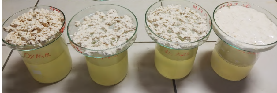
Fig. 4.3: Flocculated biomass after filtration (Petri dish) and its liquor (beaker above). Leftmost sample contains no added salt, others had 1%, 2% and 3% of added NaCl, respectively.
