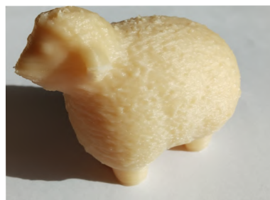
Fig. 4.35: 3D printed object made from PHB. The polymer came from soap-based digestion and was stabilized with 2 % succinic anhydride before melt processing
