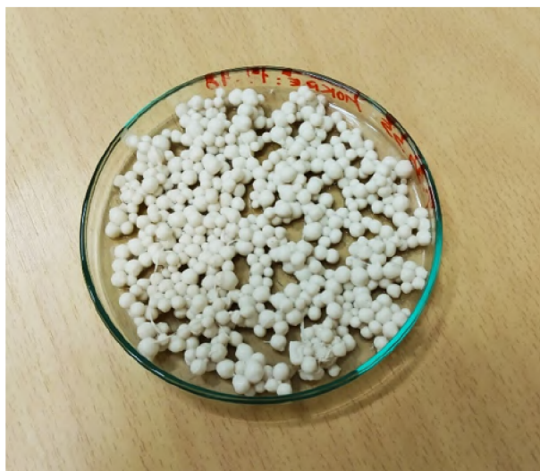
Fig. 4.5: Spherical flocks obtained by dropping alkaline biomass gel to acid solution
