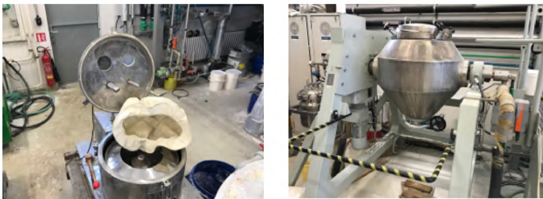
Fig. 4.13: Drum centrifuge and drum vacuum drier for flocks separation and drying
