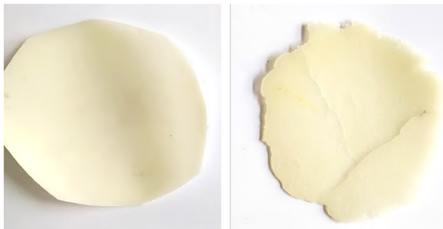
Fig. 4.31: PHB samples after melting at 190 °C/5 min and cooling. Left: commercial PHB, right: PHB obtained by soap-based digestion. The sample spontaneously cracked upon cooling.
