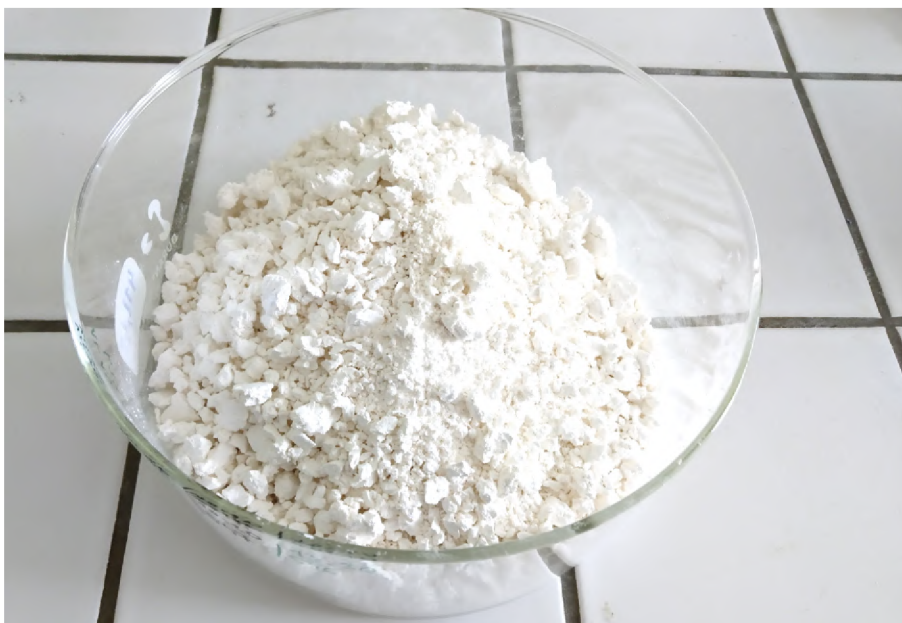
Fig. 4.26: PHB isolated by soap-based digestion
