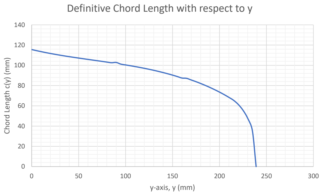
Figure 21 A graph of wing's Definitive Chord Length vs Y : Derived from the Geometry Acquisition section
