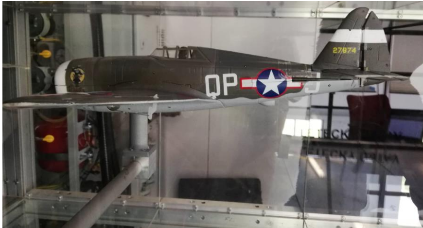
Figure 78 The model mounted in the test chamber during testing at AoA of 0 degrees
