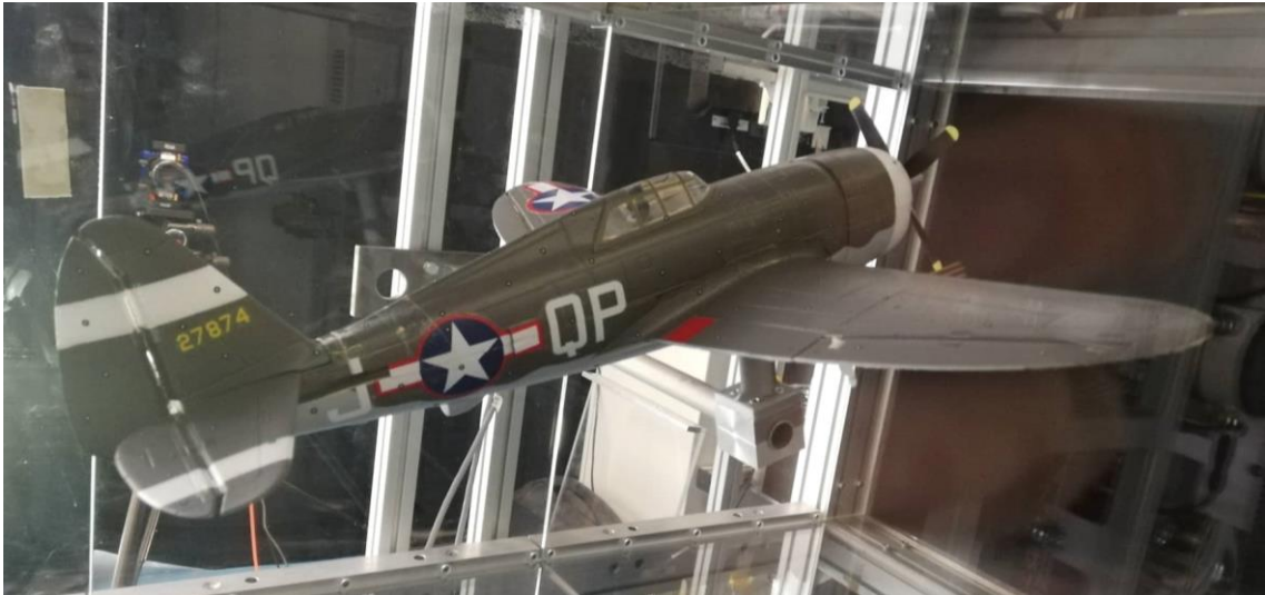
Figure 76 The model mounted in the test chamber before testing at AoA of 17 degrees
