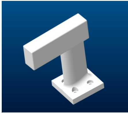
Figure 73 CAD Model of the intermediate fixture for balance mounting
