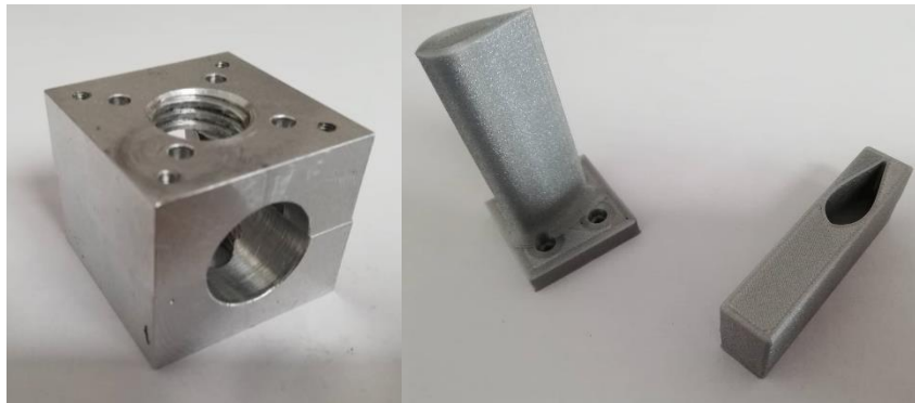
Figure 74 The clamp (left) used and the two 3D printed parts (right) of the intermediate fixture.
