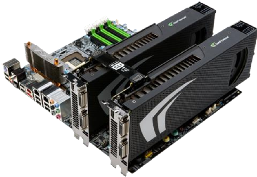
Figure 1 - Two graphics cards from Nvidia connected via SLI.
