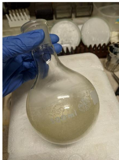
Figure 6 Round-bottom flask with bacteria lyophilate coating on inner wall.
