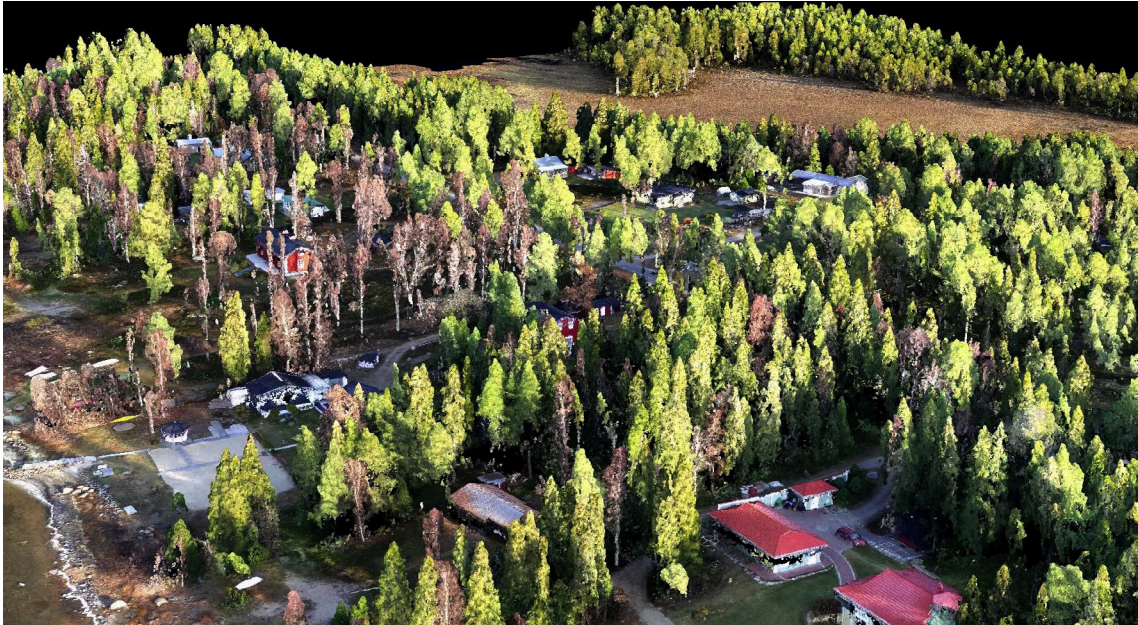
Fig. 6. Visualisation of very high-density coloured image-based point cloud representing boreal forest stand and several buildings, generated from UAV-borne RGB images. Source: Nyström (2015).
