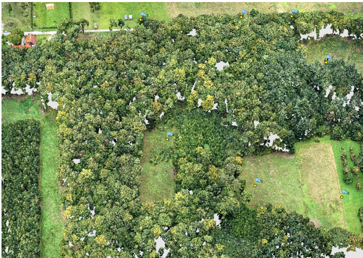
Fig. 43. A high quality surface representation in the form of the Dense point cloud in Agisoft PhotoScan.
