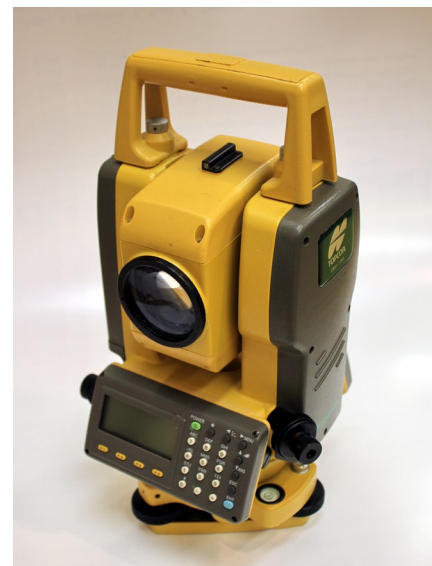
Fig. 16. Total station TOPCON Green Label GTS-105N.
