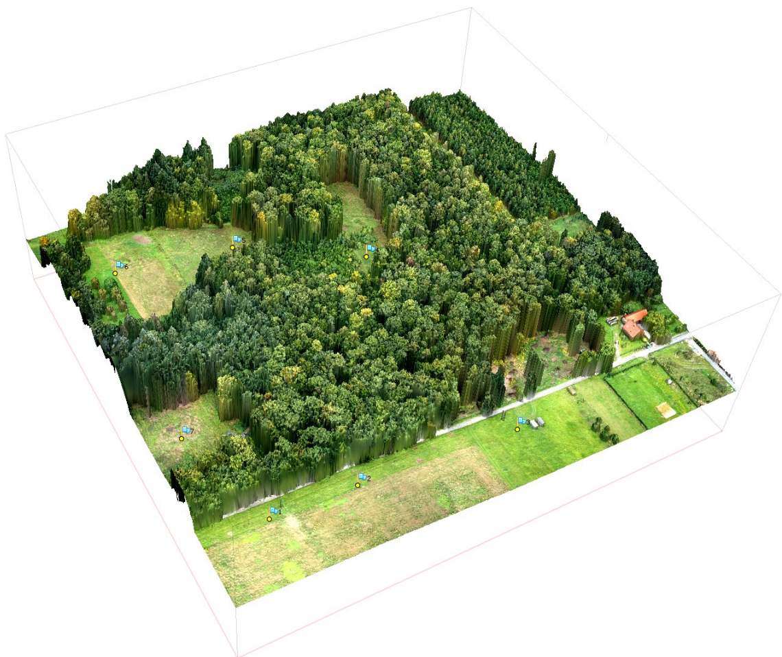
Fig. 45. Mesh model - a 3D polygonal mesh with texture representing the object surface based on the dense point cloud. Generated and displayed in Agisoft PhotoScan software.
