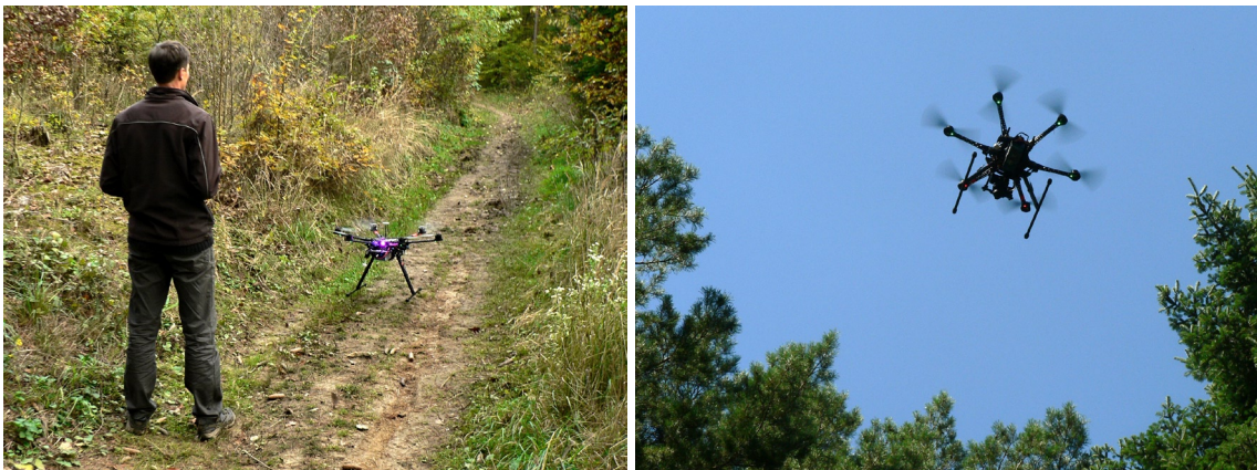
Fig. 34. The pilot and the DJI S800 just before the takeoff (left) and the machine on another site rising above the forest stand, heading to the given position when starting a new mission (right).
