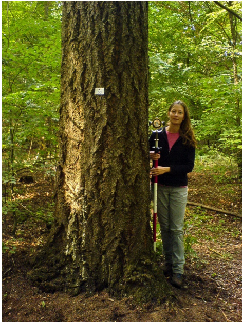
Fig. 26. Geodetic measurements of the tree trunk centre with a total station using a horizontal offset.
