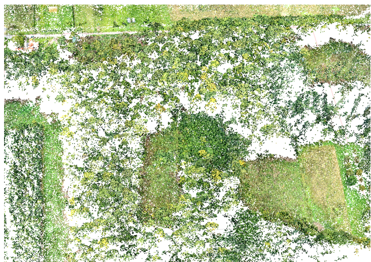
Fig. 41. Sparse point cloud as a result of image alignment in Agisoft PhotoScan.
