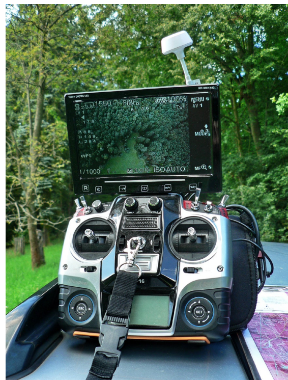
Fig. 29. Graupner MX-20 HoTT Transmitter with attached display showing live image and telemetry UAV data.
