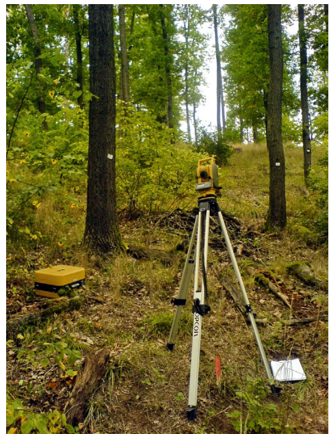
Fig. 24. The total station situated above the wooden stake just at the plot centre, ready for measurements of the positions of all the trees being thoroughly examined.
