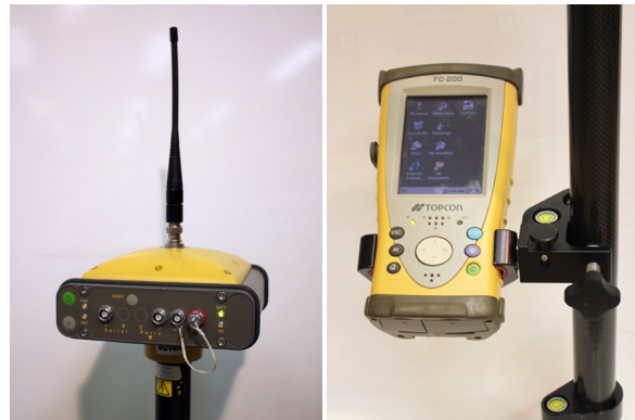
Fig. 18. TOPCON HiPer Pro GNSS receiver (left) and TOPCON FC-200 Windows field Bluetooth controller (right).
