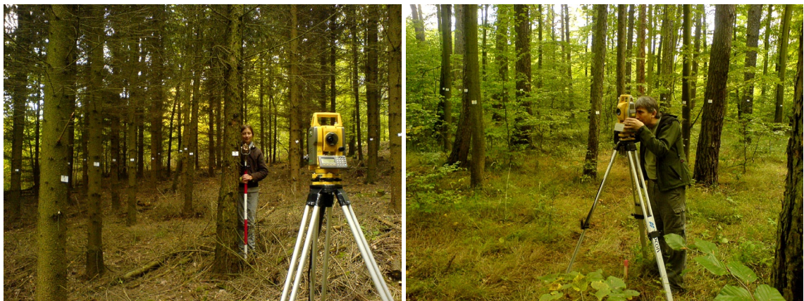
Fig. 25. Geodetic measurements of the positions of the trees on different study plots.
