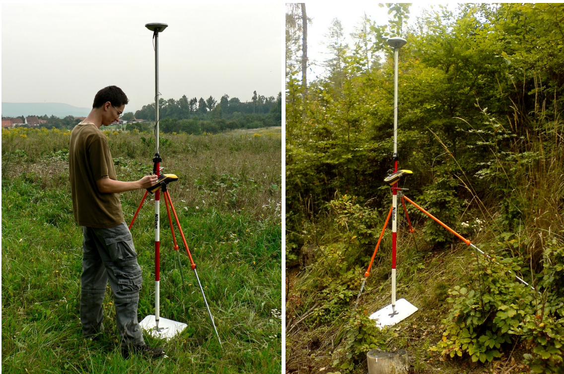
Fig. 33. Operator setting the GNSS receiver TRIMBLE GeoExplorer 6000 for iterative measuring of the accurate position of a GCP marker (left) and the same device positioned above a marker situated on a very steep terrain (right).
