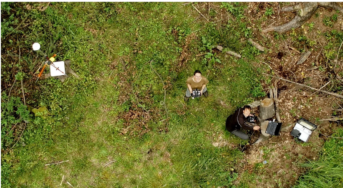
Fig. 35. The pilot (person on the right) and the assistant watching the UAV during the flight mission. A GNSS device measuring the position of a GCP marker can be seen on the left.
