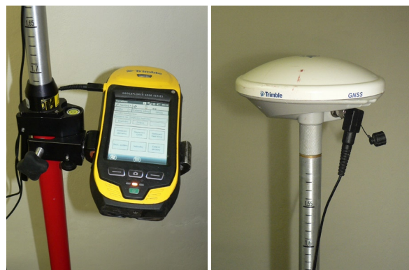
Fig. 19. Trimble GeoXH 6000 GNSS receiver handheld (left) and Trimble Zephyr 2 broad frequency tracking antenna (right).
