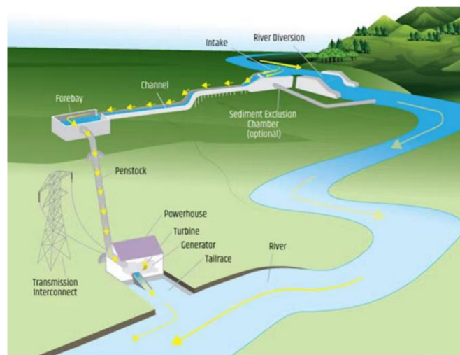
Figure 3.6: Schematic of run of river small hydro power plant (Source – US Department of Energy)
