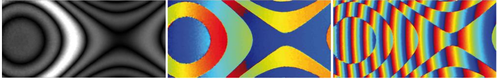
Figure 3.28: (left) Magnitude map; (middle) phase map with almost no phase drift. Phase jumps correspond to zeroes in the magnitude map; (right) phase map including a phase drift.
