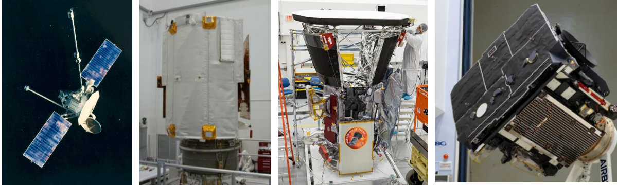
Figure 5-4 Comparison of various sunshades. From left to right: Mariner 10 [44], MESSENGER [43], Parker Solar Probe [45], Solar Orbiter [46]
