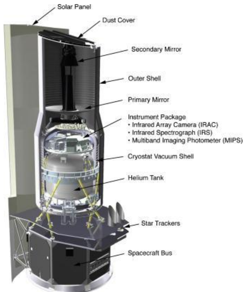
Figure 8-1 Cutaway view of the Spitzer cryogenic telescope assembly showing the details of its mounting to the spacecraft bus and internal details of the structure. Conductive isolation from the bus is accomplished using struts (yellow). [76]
