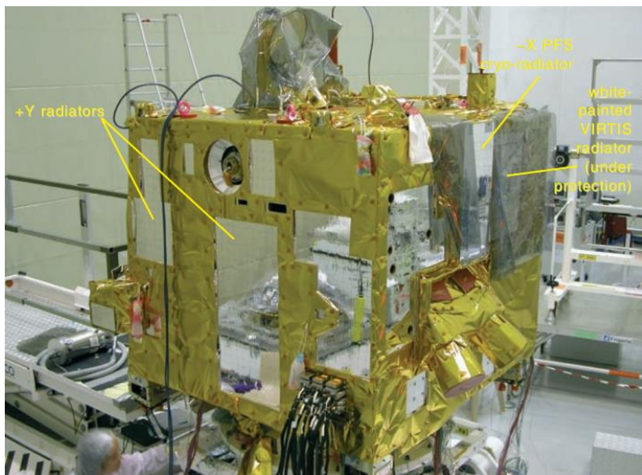
Figure 4-3 External components of the TCS of Venus Express. [28]
