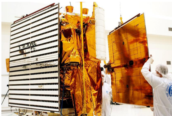
Figure 5-5 Messenger's solar panel installation. Note the alternating rows of solar cells (dark) and OSRs (metallic white). [49]
