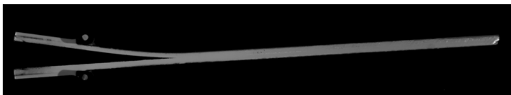
Figure 6.1: DCB specimen opening before crack growth
