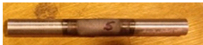
Fig. 39 Diffusion welded Sample 5 under the mentioned parameter
