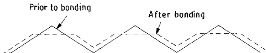
Fig.8. Surface structure before and after welding [14]
