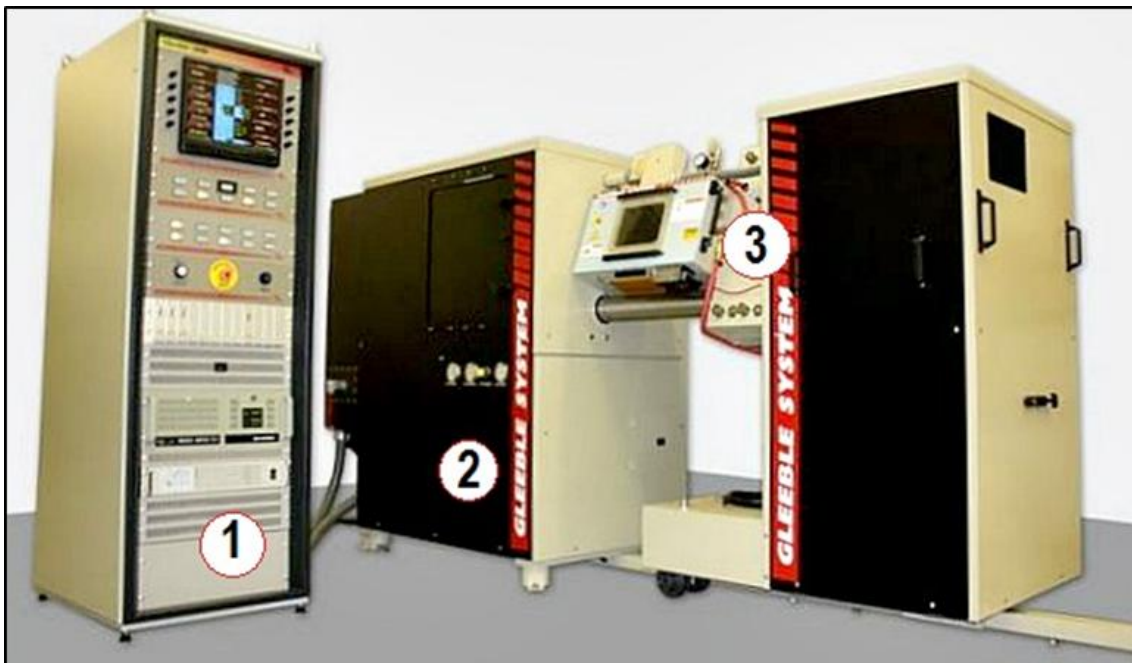
Fig. 13. Basic Gleeble 3500 simulator assembly. 1- Console; 2- Load unit; 3 – Pocket Jaw
