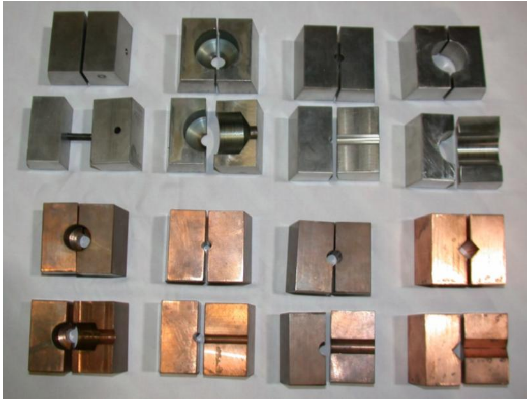
Fig. 17 Jaws with partial and complete contact made of copper and X5CrNi18-8 steel intended for different shapes of test samples
