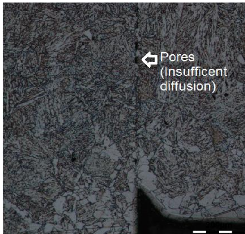
Fig.34. Microstructure 30mins holding time at 1125 °C
