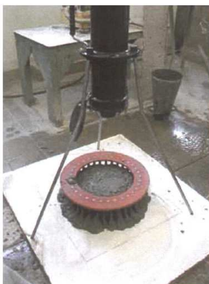
Obr. 4-4 Zkouška Orimet + J-Ring [14]
