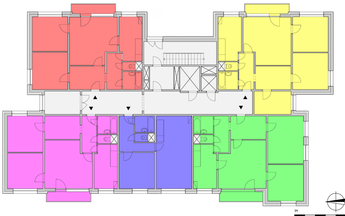
Figure 25. Layout of a residential floor in Koniklecová 4 block-of-flats. Individual flats are highlighted by different colours. (Mørck, 2017)
