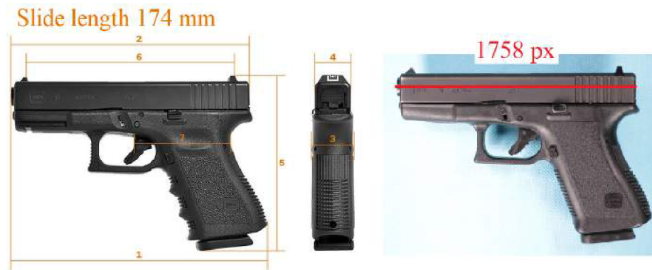
Figure 2.8: Image of G19 Glock with length slide (left). Image acquired by the device with the measured length of the slide in pixels (right).
