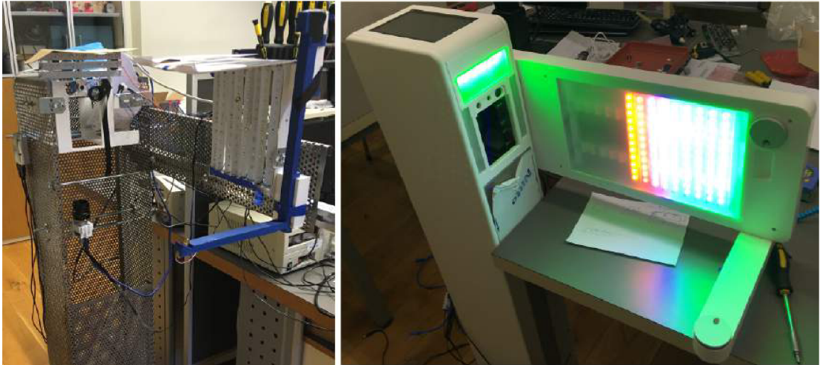
Figure 2.17: Custom build case with updated components and placement (left), final prototype with contracted case (right).
