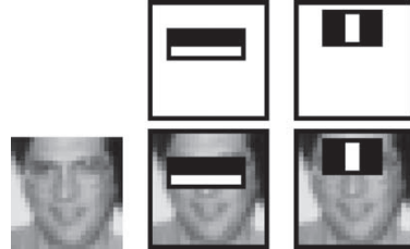
Figure 3.6: First and second Haar features selected by AdaBoost in Viola and Jones detector. The first feature exploits difference of intensity between region of eyes and region of upper cheek. Taken from [32]
