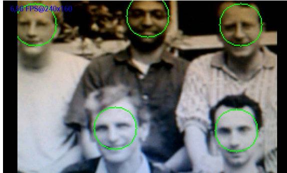
Figure 7.2: Android detection is set to detect only specific sizes of faces, therefore its hard to compare results.
