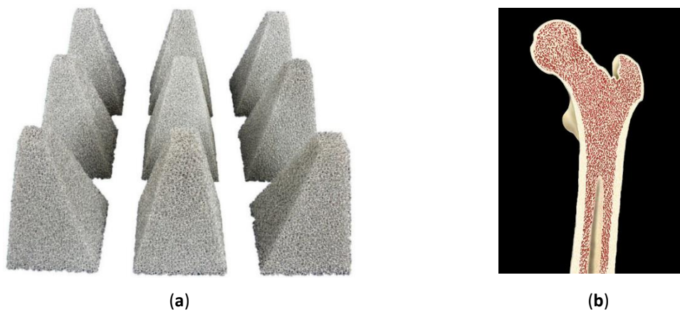
Fig. 1.1. (a) Absorbers of impact energy from metal foam [4]; (b) inner structure of bone [5]
