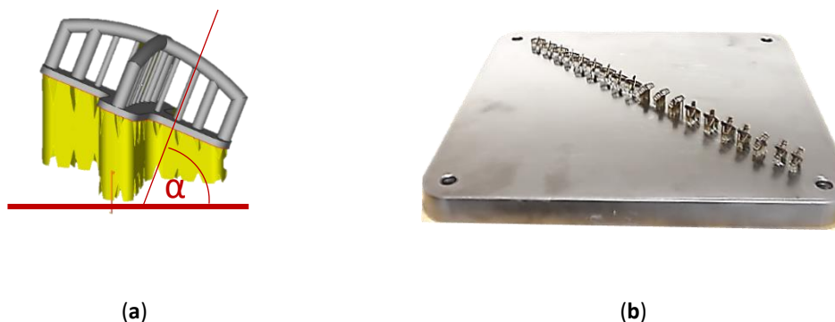
Fig. 5.6. (a) Orientation of specimen with support structures; (b) Produced specimen fixed on the platform
