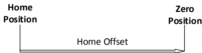
Figure 11 Homing mode - displacement of zero position [4]
