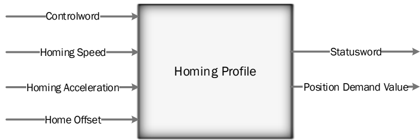
Figure 10 Simple homing profile representation
