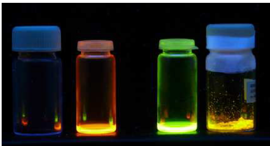
Figure 5 Sample DPP U115 and DPP U116 under UV light in solid and liquid state.
