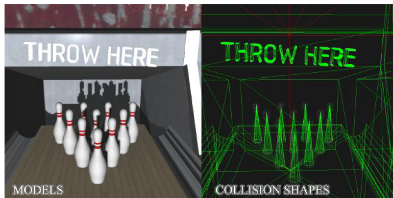
Figure 4.3: The approximation of a pin collision shape is a cone.
