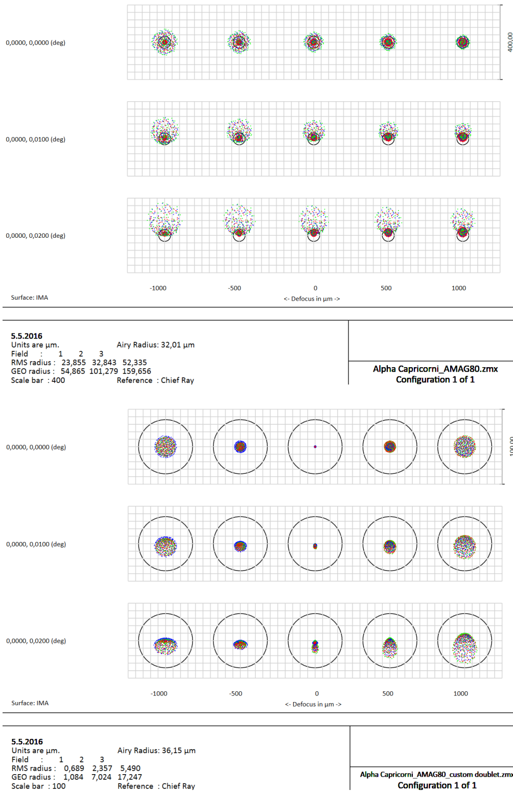
Figure 104: Spot diagram comparison of a telescope with commercial (upper) and custom (lower) doublets.
