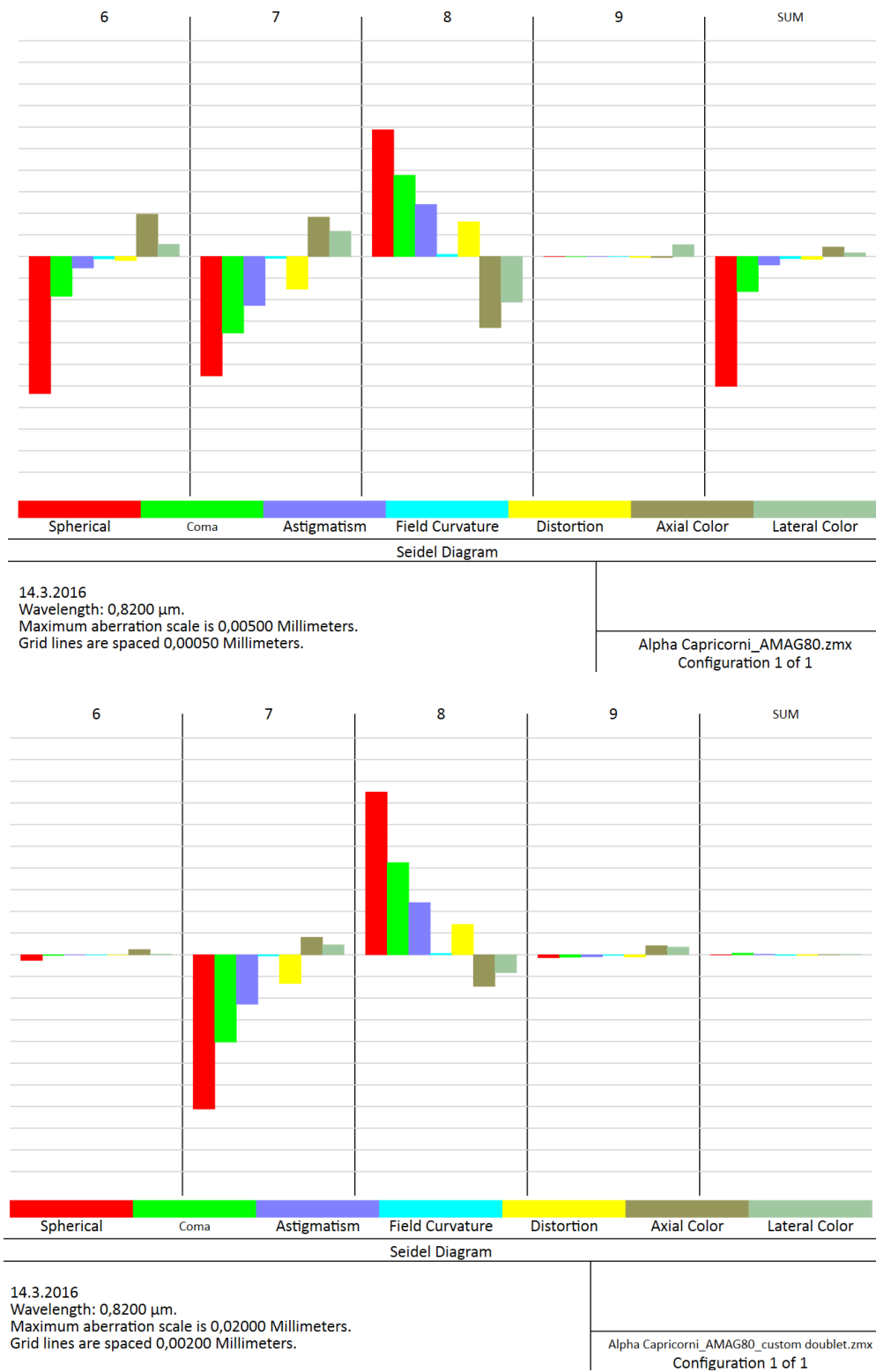
Figure 103: Seidel aberration comparison of a telescope with commercial (upper) and custom (lower) doublets.
