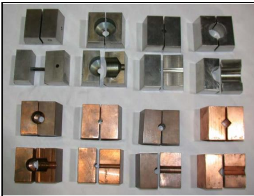
Figure 15 Full and partial contact jaws of different shapes
