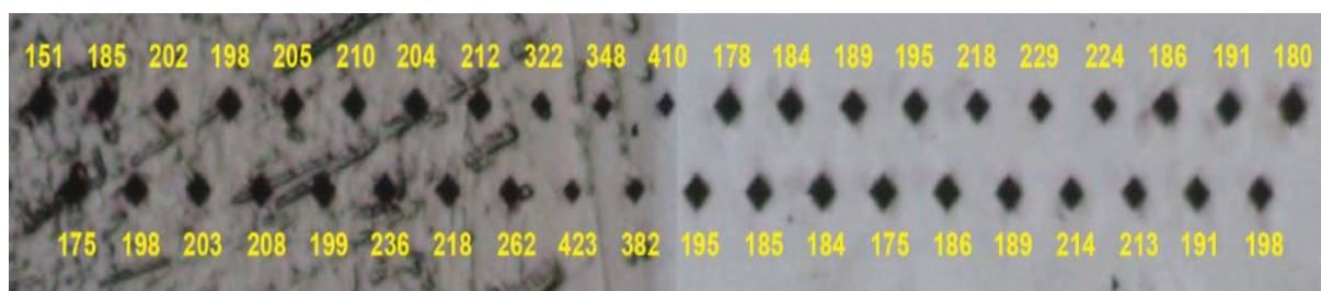
Figure 33 Micro-hardness HV 0.1 distribution over the diffusion welded joint in furnace of sample no. 5
