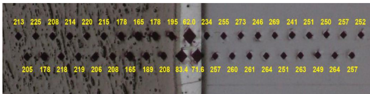
Figure 30 Micro-hardness HV 0.1 distribution over the diffusion welded joint of sample no. 3 (T820_F0.7_t20)
