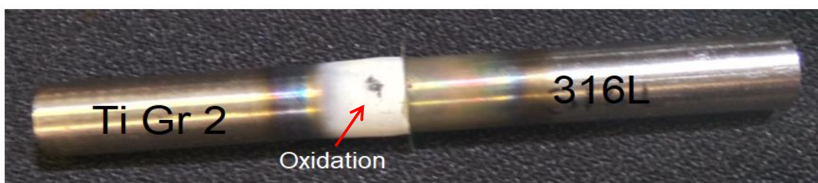
Figure 24 Oxidation on the surface of titanium
