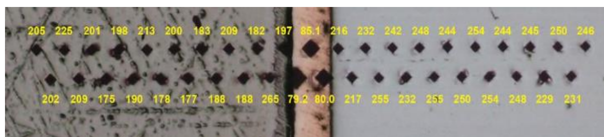
Figure 40 Micro-hardness HV 0.1 distribution over the diffusion welded joint of sample no. 3 (T820_F0.7_t60)
