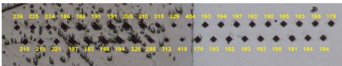
Figure 42 Micro-hardness HV 0.1 distribution over the diffusion welded joint in furnace of sample no.4
