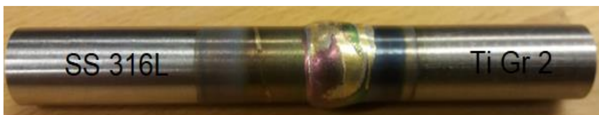
Figure 36 Higher deformations on the titanium side of sample no. 1 (T870_F0.5_t40)
