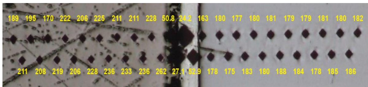
Figure 35 Micro-hardness HV 0.1 distribution over the diffusion welded joint in furnace of sample no. 6
