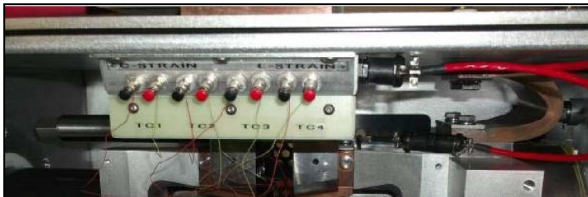
Figure 13 Four thermocouple channels and side outlet for pyrometer [21]
