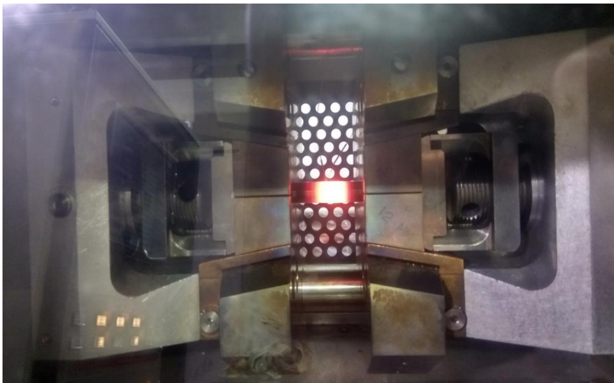
Figure 22 Diffusion bonding operation during holding time
