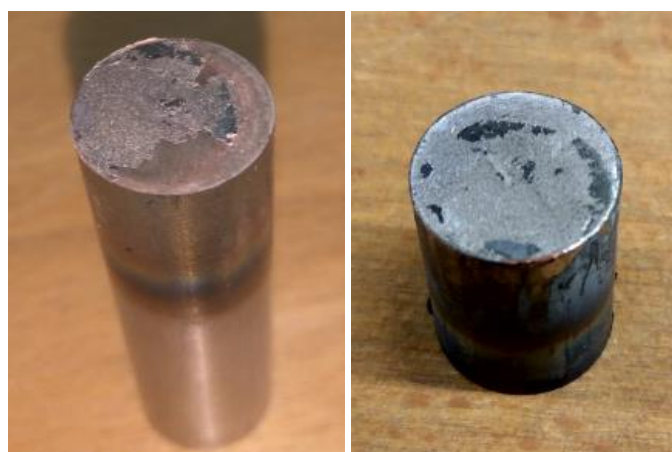
Figure 37 broken sample no. 2 (T850_F0.5_t30)
