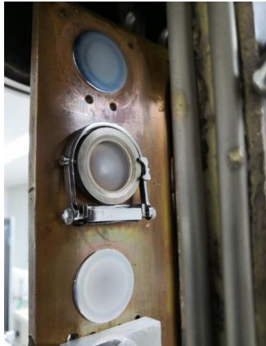
Figure 22: Securing mechanism of a collector plate. [2]
