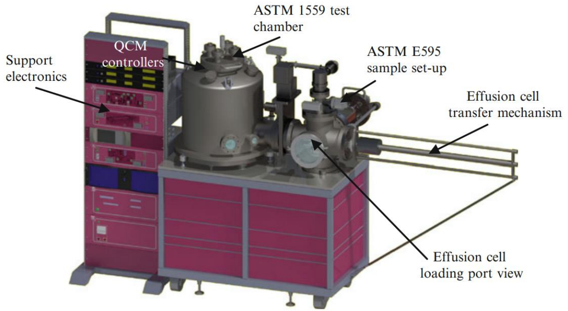
Figure 24: ASTM E-595 and ASTM E-1559 testing device. [16]
