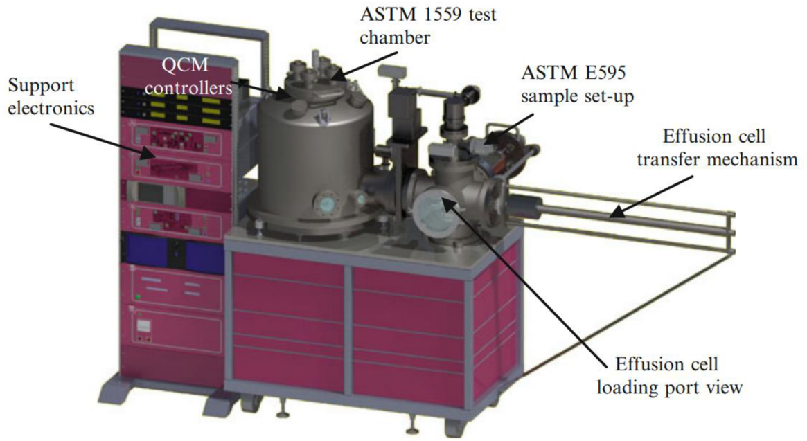
Figure 24: ASTM E-595 and ASTM E-1559 testing device. [16]
