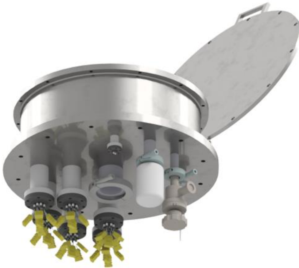
Figure 69: Bottom of the vacuum chamber will all connections modeled.
