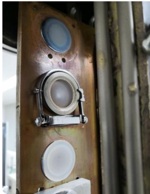
Figure 22: Securing mechanism of a collector plate. [2]
