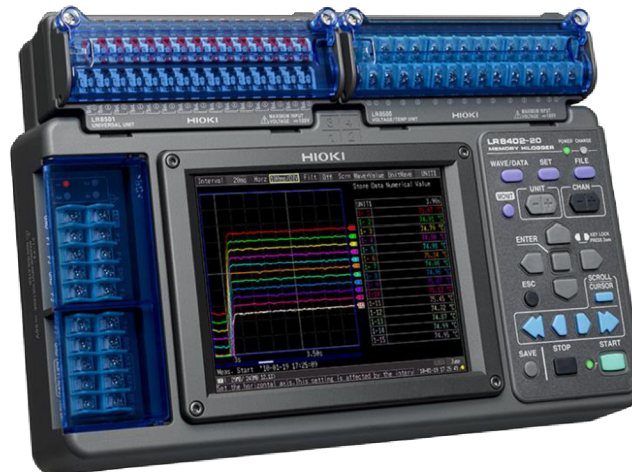
Figure 44: Hioki LR8400 data logger. [40]
