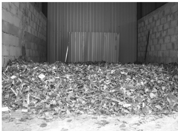
Fig. 8. Layer of cherry tree chips in the drying chamber of biomass dryer
