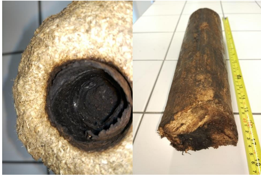
Figure 25. The clog of the channel of briquette (left image) and fragment of briquette after detonation (right picture).
