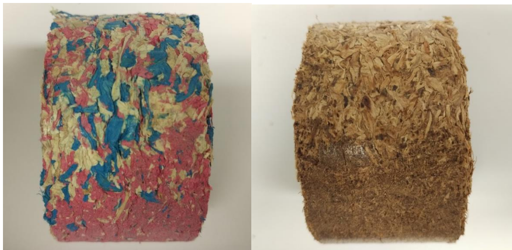
Figure 47. The result of the segregation of particles in the structure of briquettes
