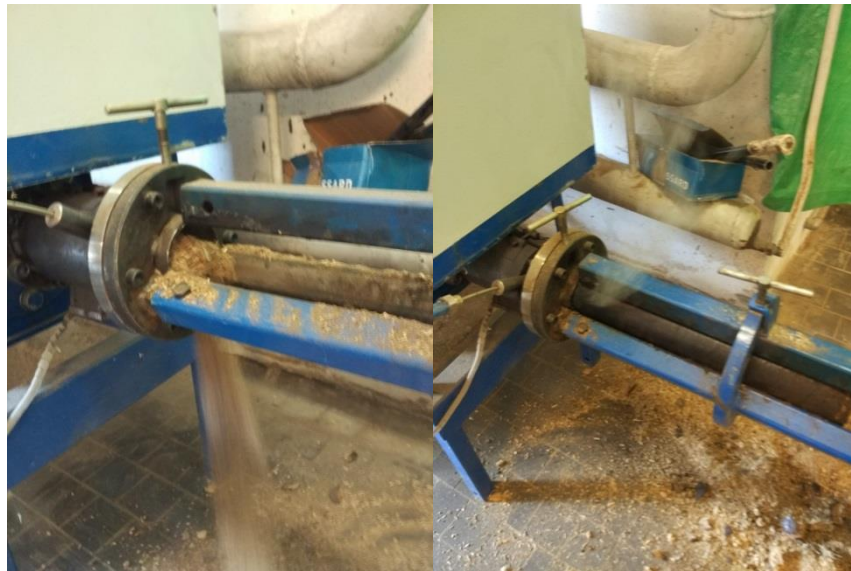
Figure 24. Work of the press at the high speed and the low speed (optimal speed).
