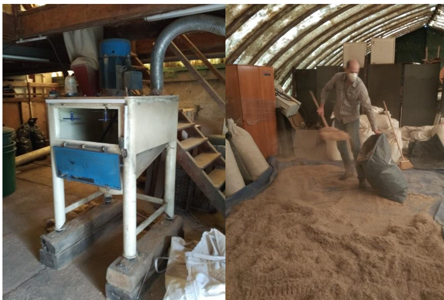
Figure 7. Hammer mill STOZA ŠV 15 (left image) and process of the drying of biomass (right image)
