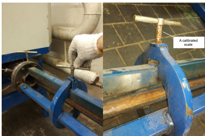
Figure 26. The adjustment of clamping screws of the cooling line.
