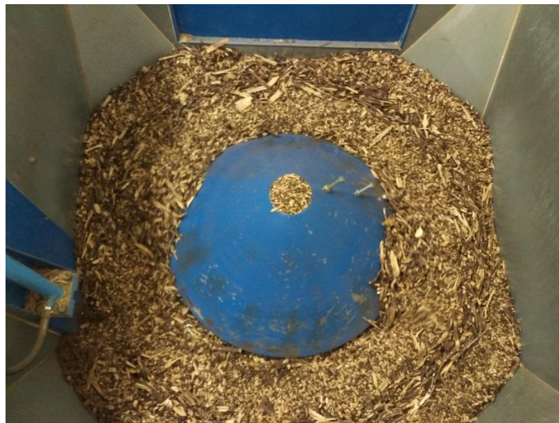
Figure 49. The process of biomass agitating in the hopper of HBP
