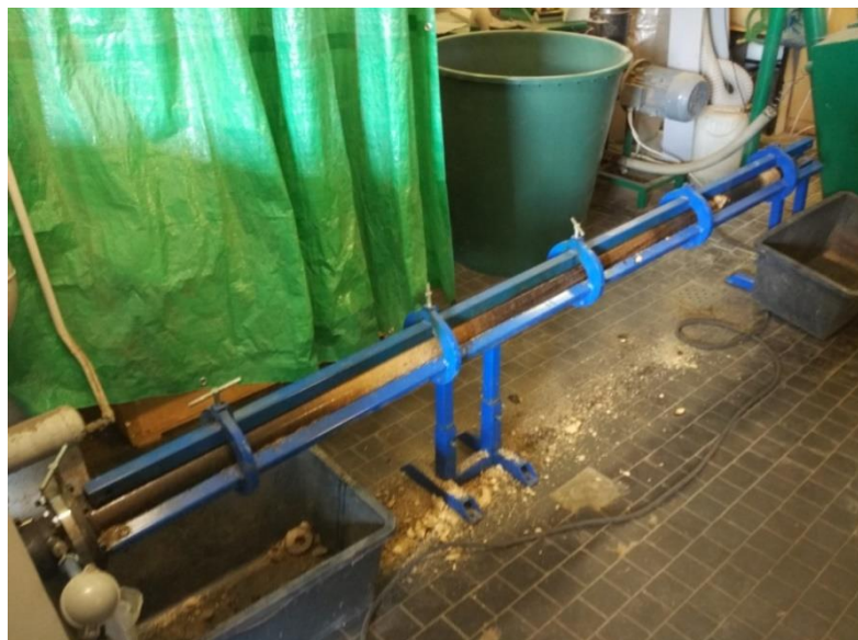
Figure 22. The view of produced briquettes obtained in the result of unsatisfactory work of transducer of the heat
