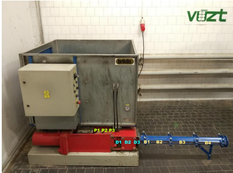
Figure 12. Areas of the measurements of the temperature during briquetting on HBP
