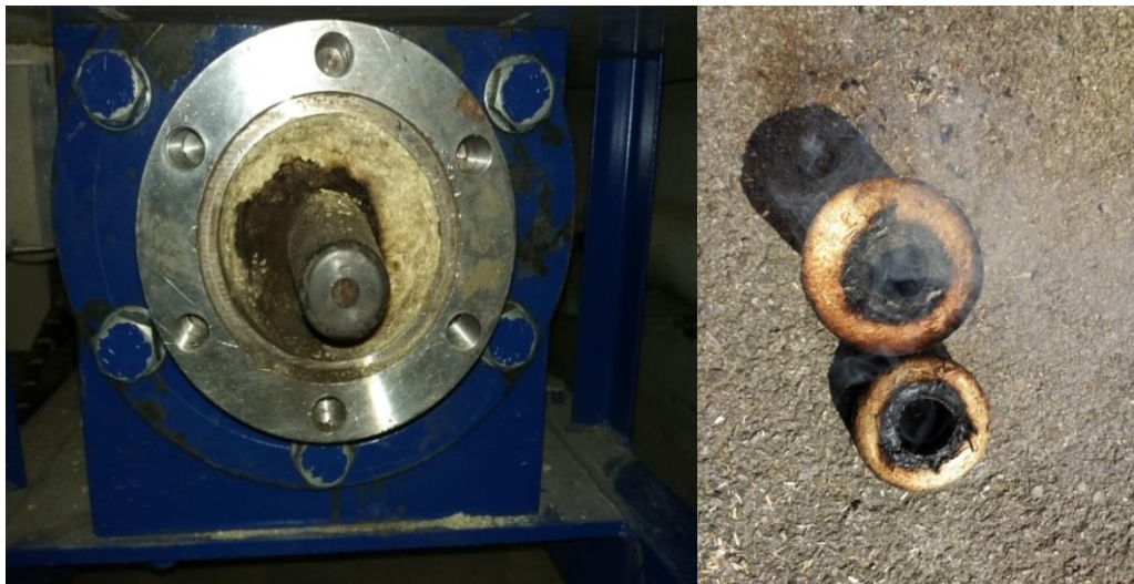
Figure 23. The impact of high temperature (inside the briquettes) obtained in the result of high friction between screw and biomass
