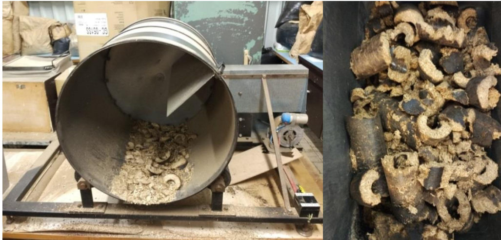
Figure 27. The influence of the high moisture on the quality of briquettes
