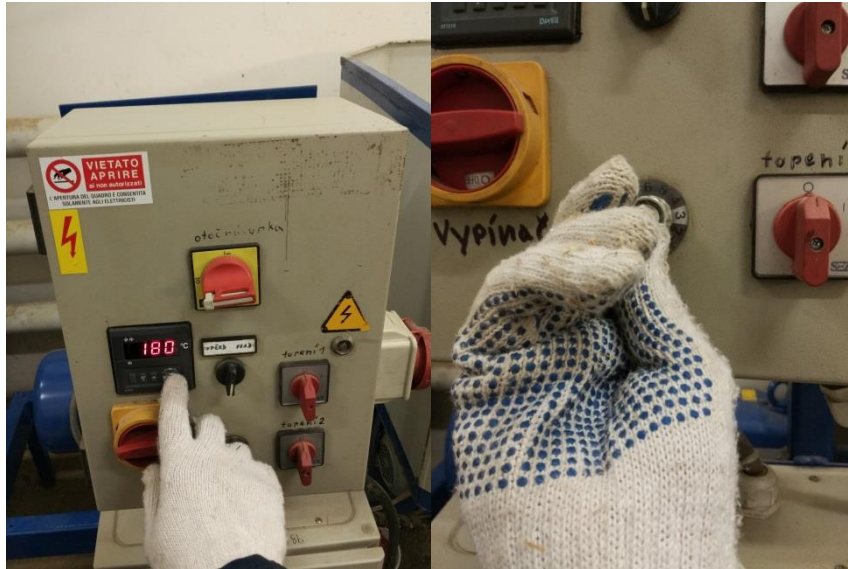
Figure 19. Setting up of the working temperature (left image) and selecting the rotation speed of the pressing screw (right image)
