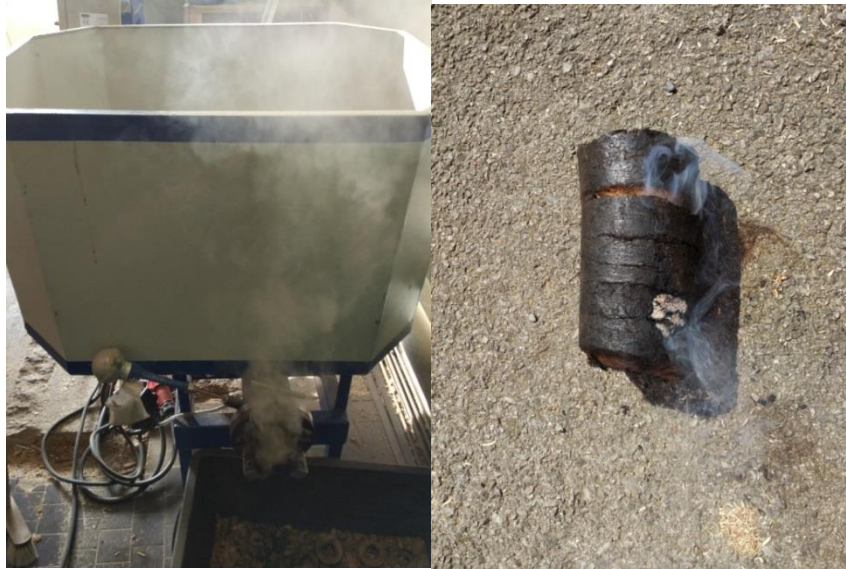
Figure 21. The consequences of high temperature excess on the production of the briquettes
