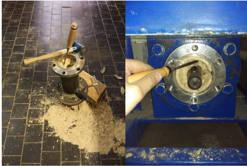
Figure 20. The laborious cleaning process of the forming and heating die.
