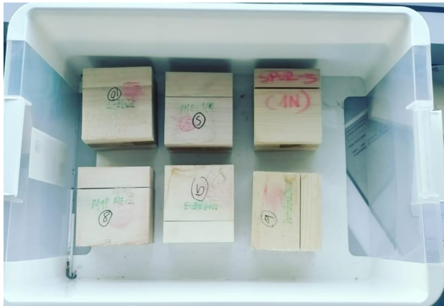
Figure 14: Water absorption and thickness swelling test
