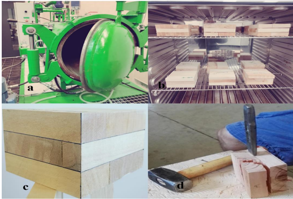
Figure 15: Delamination test; (a) vacuum-pressure cycle, (b) drying of specimen in hot air oven, (c) measurement of delamination, (d) wood failure evaluation
