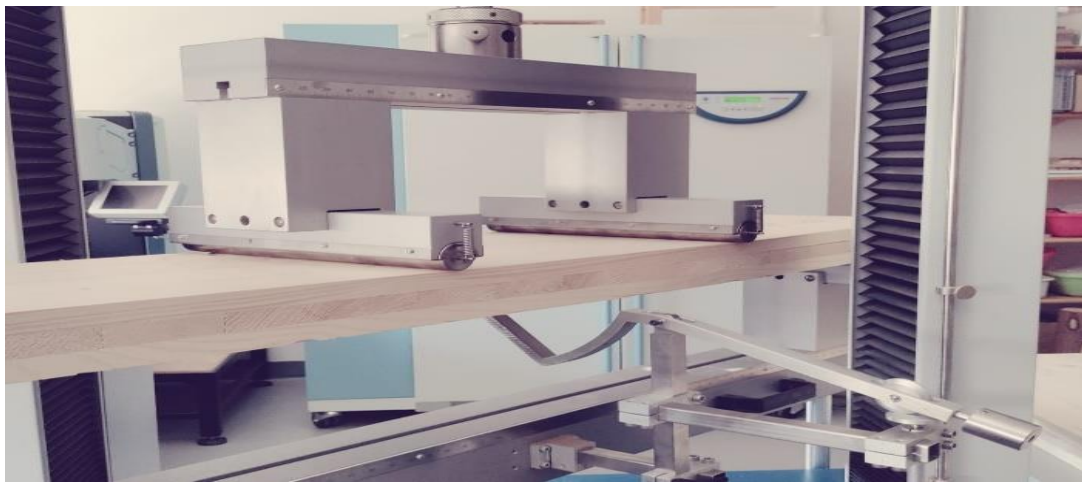
Figure 17: 4-point bending test CLT panels
