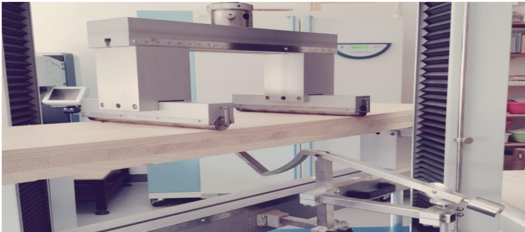
Figure 17: 4-point bending test CLT panels
