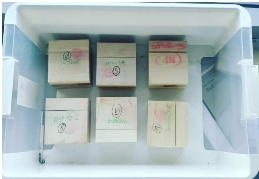
Figure 14: Water absorption and thickness swelling test
