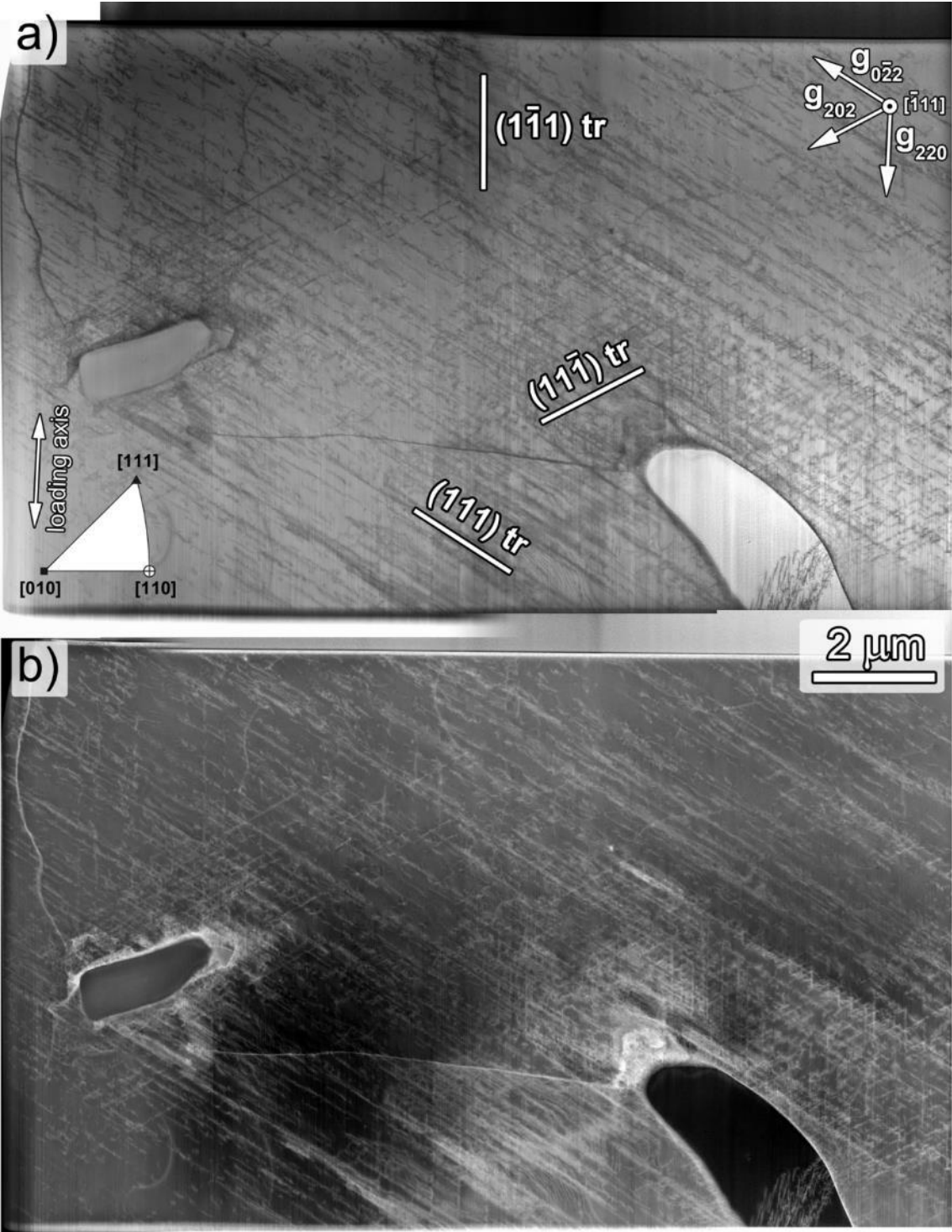
Figure 11.2: (a) BF-STEM diffraction contrast image showing dislocation structure formed after cyclic loading with total strain amplitude 0.35% at room temperature. View direction is along the zone axis [\bar{1}11] . Loading axis corresponds to vector [110] when taken with respect to the grain orientation. (b) ADF-STEM image.
