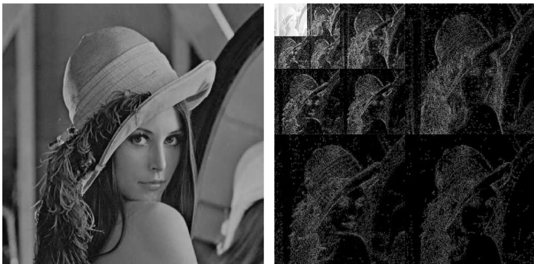
Figure 1.7: Two-dimensional separable wavelet decomposition of Lena image, using CDF9/7 wavelet and J = 3 . Logarithm of absolute values of coefficients is displayed. The representation is not expansive because of both symmetrical filters are symmetrical boundary extensions.
