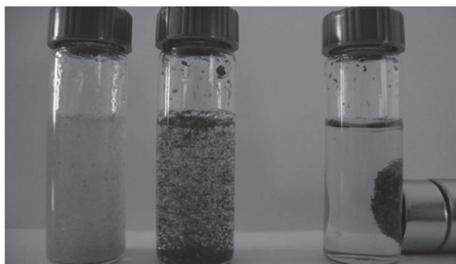
Figure 4. Appearance of original barley straw suspension (left), suspension of straw after magnetic modification (middle) and demonstration of magnetic separation of magnetically modified straw (right).
