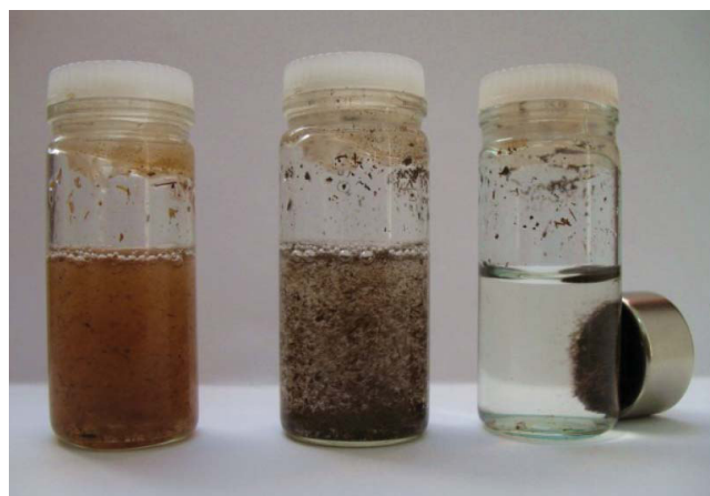
FIGURE 1 Appearance of native spent rooibos biomass suspension ( left ), suspension of rooibos biomass after magnetic modification ( middle ), and demonstration of magnetic separation of magnetically modified rooibos biomass ( right ).
