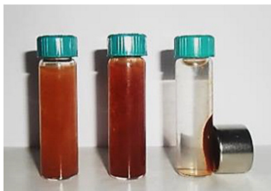
Fig. 4. A demonstration of magnetic separation of magnetically modified sheaths. Appearance of native Leptothrix sheaths suspension (left), suspension of sheaths after magnetic modification with magnetic fluid (middle) and demonstration of magnetic separation of magnetically modified sheaths (right).
