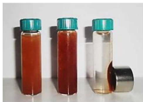
Fig. 5. Appearance of native Leptothrix sheaths suspension (left), suspension of sheaths after magnetic modification (middle) and demonstration of magnetic separation of magnetically modified sheaths (right). Almost the same appearance was observed after magnetic modification with microwave synthesized magnetite particles and with magnetic fluid.
