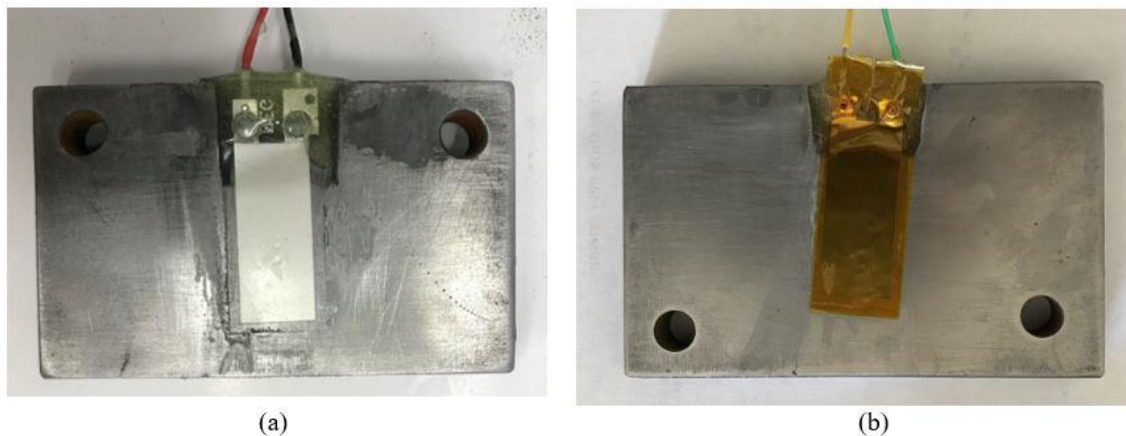
Figure 3.11: (a) MSI PVDF sensor (12 mm × 30 mm), (b) TUL PVDF sensor (12 mm × 30 mm)
