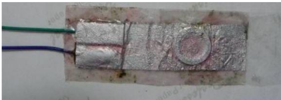
Figure 2.13: Flexible thin-film single point force sensor from PVDF film [15].
