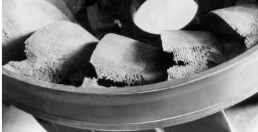
Figure 1.2: Major cavitation damage to the blades at the discharge from a Francis turbine [35].
