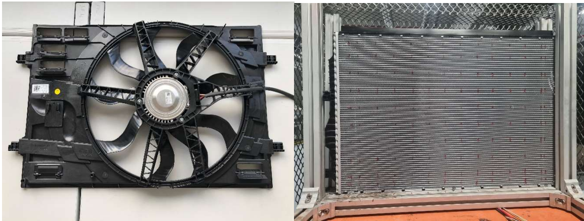
Figure 6. MQB platform cooling assembly
