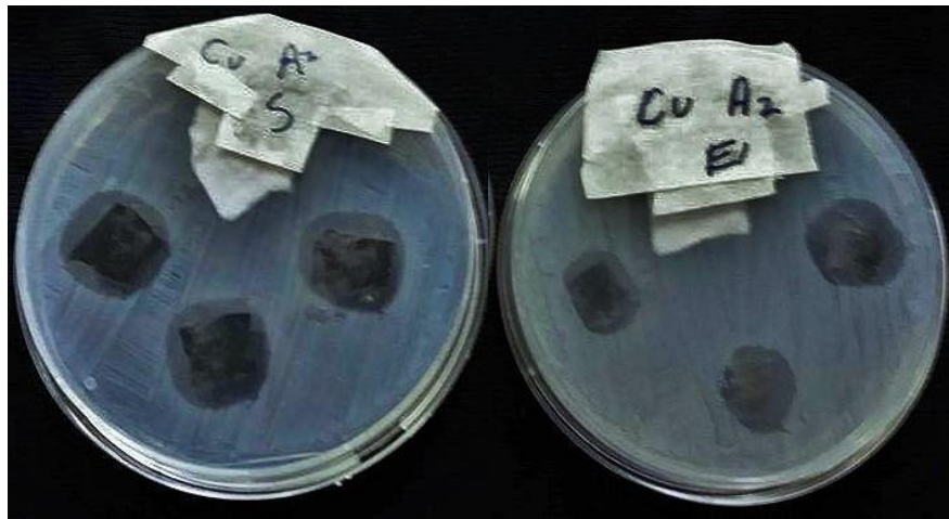
Figure 35: Zone of inhibition for copper coated cotton fabrics
