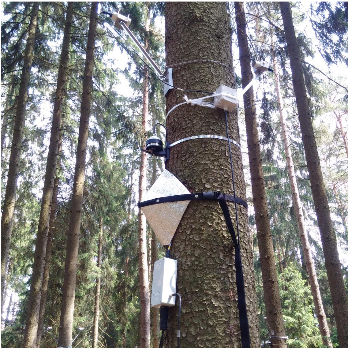
Figure 10: Example of sensors. Sap flow meter EMS81 with isolation and automatic band dendrometer EMS81 without isolation.
