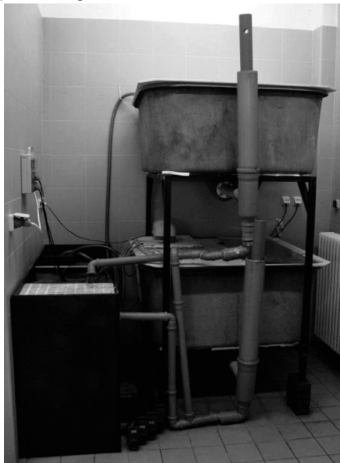
Fig. 11. Recirculation aquaculture system for rearing of African sharptooth catfish broodstock (aquarium room IA FFPW USB). Photo by B. Drozd
