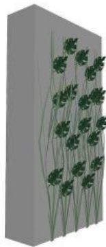
Direct green façades
