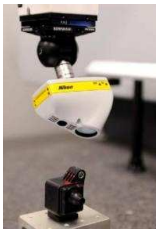
Obr. 3.15: Nikon LC15Dx v praxi a jeho princip [30]
