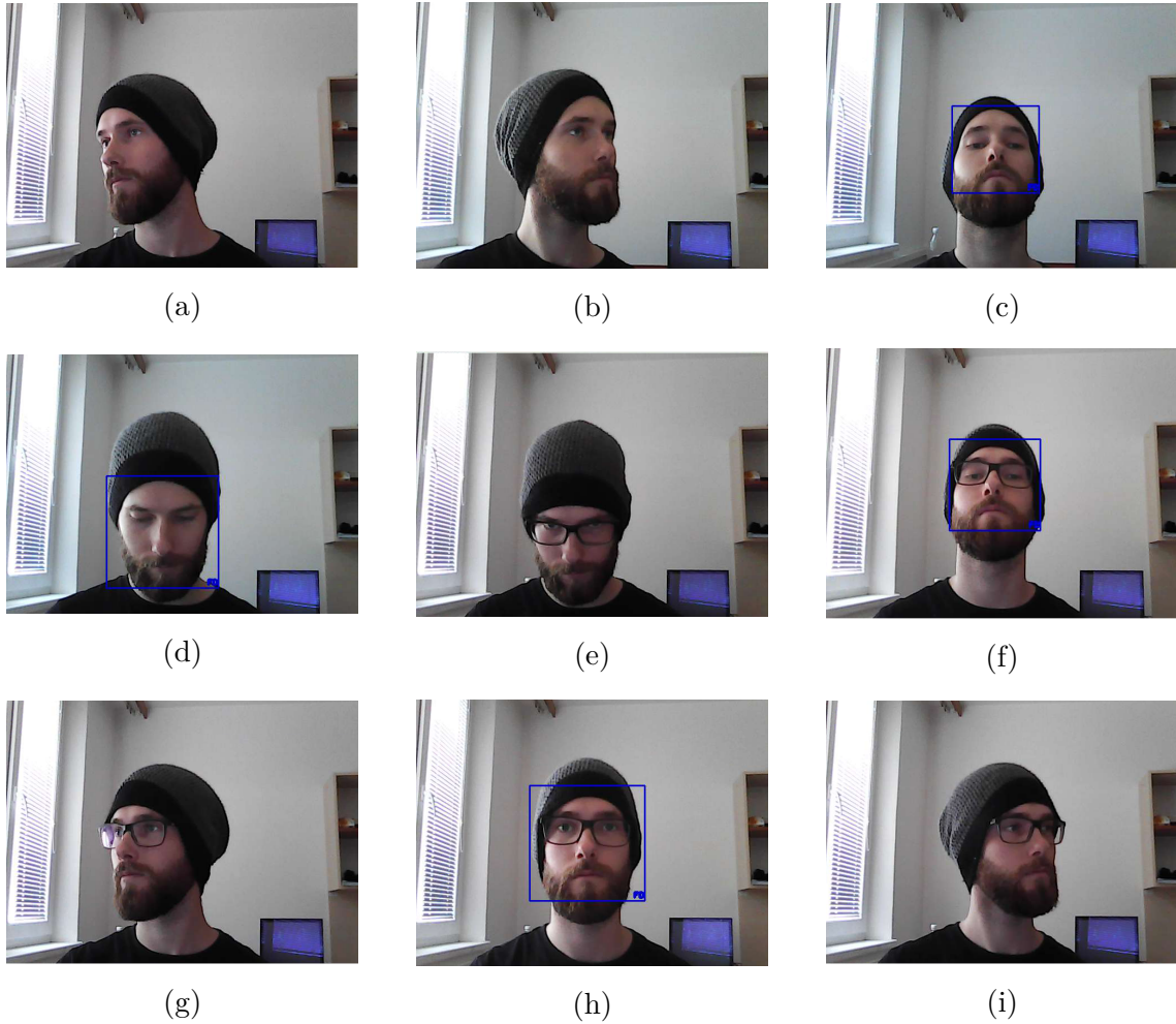
Fig. 4.6: Results of LBP face detection on face with cap(a-d) and glasses(e-i)
