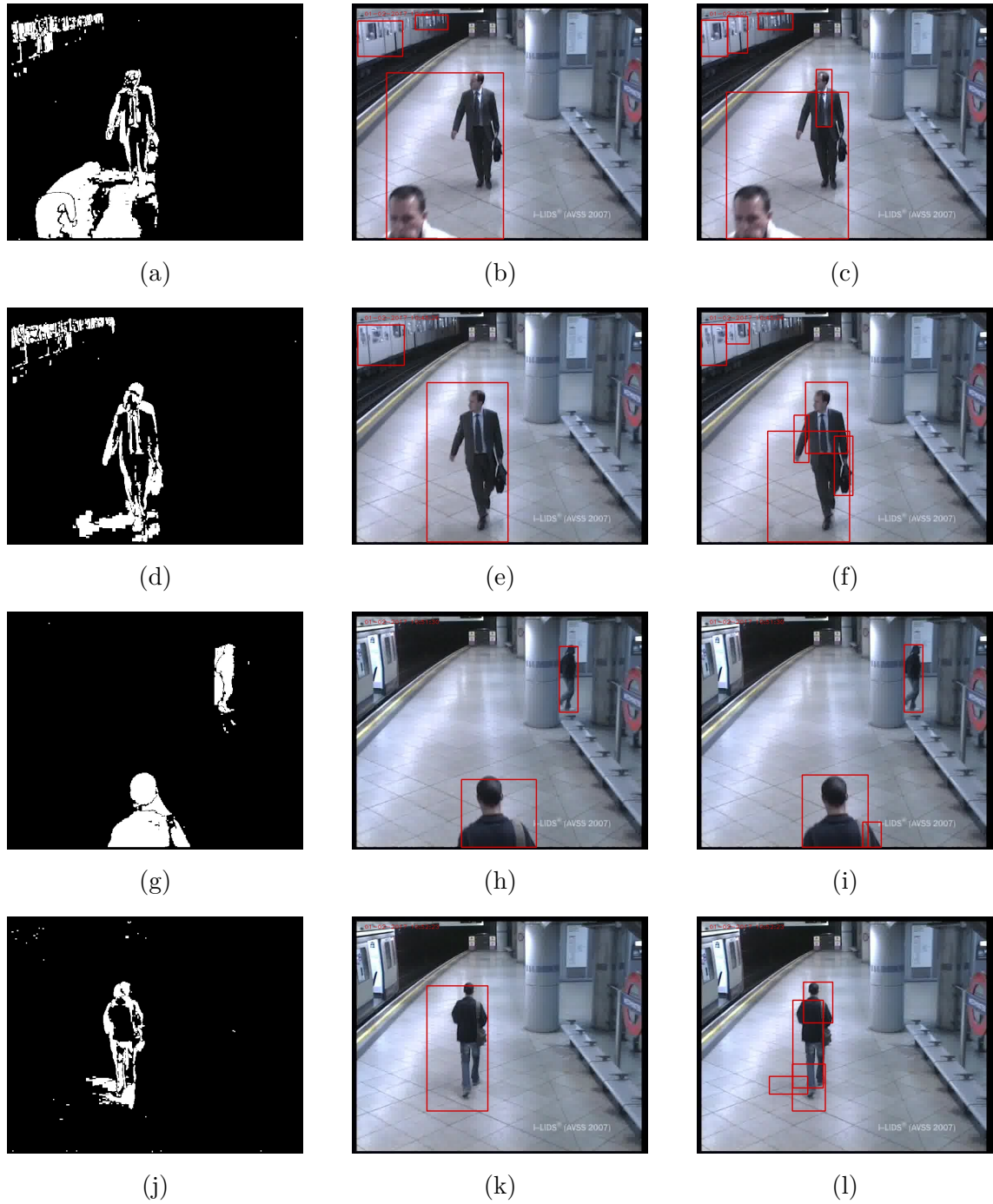
Fig. 4.3: Motion detection: metro station
