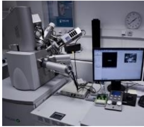
Figure 7.2.1: Dual-beam scanning electron microscope TESCAN Lyra 3 XMU FEG-SEM.
