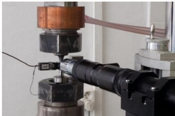
Figure 7.1.1: Long focal distance light microscope Navitar equipped with Olympus DP 70 high resolution camera.
