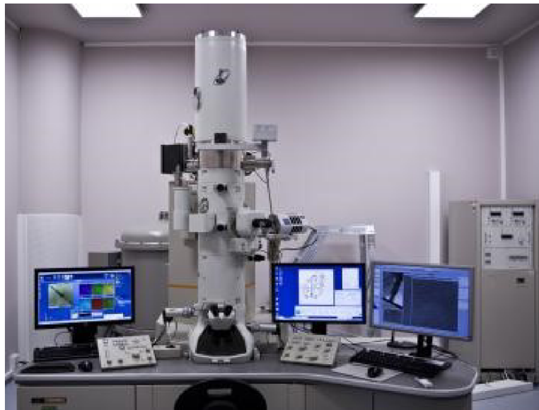
Figure 7.3.1: Transmission electron microscope JEOL JEM-2100F equipped with STEM, HAADF and EDS detectors.
