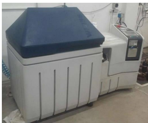
Obr. 83 Solná komora WEISS SC450
